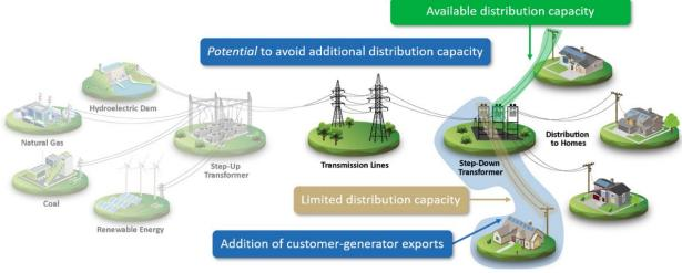
Figure 4.10 Electric grid schematic identifying localized distribution capacity
