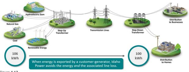
Figure 4.12 Electric grid schematic with illustrative line loss example
