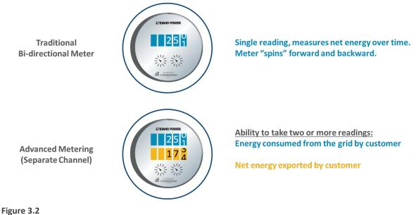
Illustration of bi-directional meter and advanced separate channel meter
