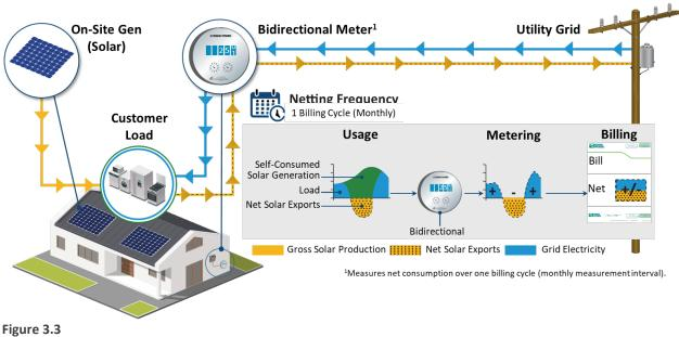
Net Energy Metering schematic
